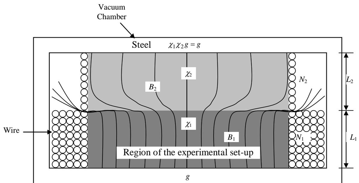
Fig. 3 – Cross-section of the vacuum chamber showing the magnetic fields  $B_1$  and  $B_2$ .
