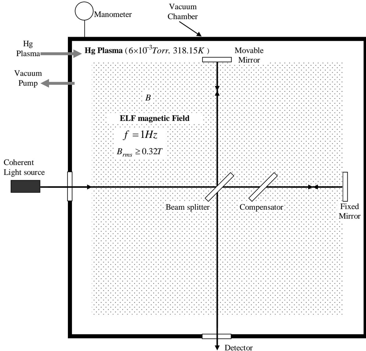
Fig. 2 - *The modified Michelson-Morley experiment. The air is substituted by Hg plasma at  $6 \times 10^{-3} \text{ Torr}$  and  $318.15 \text{ K}$ , and an ELF magnetic field with frequency  $f = 1 \text{ Hz}$  and intensity  $B_{rms} \geq 0.32 \text{ T}$  is applied through this plasma, then the displacement of the interference bands should appear.*
