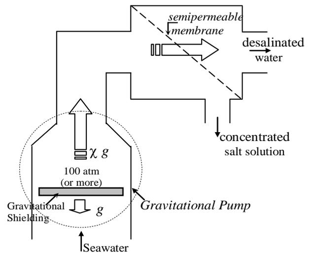
Fig. 3 – Reverse Osmosis using a *Gravitational Pump*.
