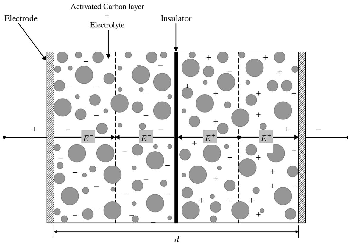
Fig. 1 – Cross-section of an *Electric Double-Layer Capacitor* (Supercapacitor) - Each *activated carbon + electrolyte* layer works as a *non-conducting plane of charge*, with density of charge  $\sigma^- = q^-/S$  and  $\sigma^+ = q^+/S$  respectively. The electric fields *through the layers*, due to these densities of charges ( $E^-, E^+$ ), are shown in the figure above.
